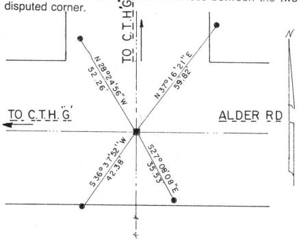
All ties to 7/8" x 30" Iron Re-bars with caps. Special County Witness Post by one of the ties. From NE Cor. to  $E^{\prime}_{4}$  Cor. S0 $^{0}$ 40'04"E, 2624.73' From NE Cor. to N $^{\prime}_{4}$  Cor. Sec. 7-31-8 S89 $^{0}$ 53'52"E, 2802.83'
