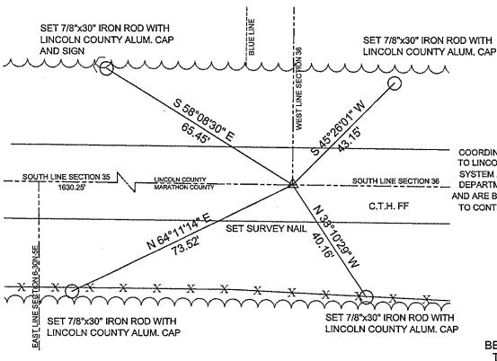
COORDINATES ARE REFERENCED TO LINCOLN COUNTY COORDINATE SYSTEM AS DEVELOPED BY THE WI. DEPARTMENT OF TRANSPORTATION AND ARE BASED ON GPS OBSERVATIONS TO CONTROL POINTS AS SUPPLIED BY LINCOLN COUNTY.
