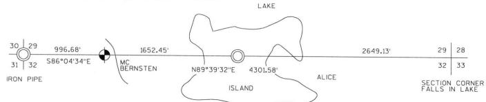
(c)(d)(e) Plan view of corner with ties to at least 4 witness monuments. If in disagreement with previously established corner, show the distances between the two corners and also indicate the ties to the disputed corner.
