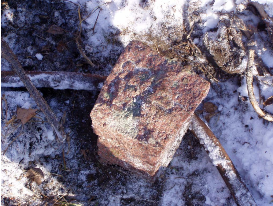
SOUTH ¼ CORNER, SECTION 33 – 6" GRANITE STONE FOUND
