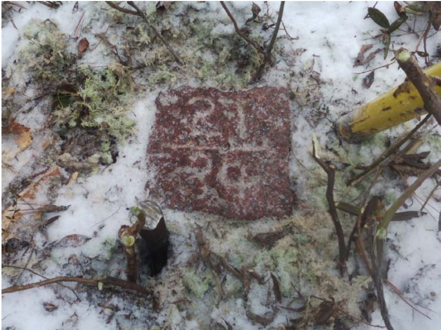
NORTH ¼ CORNER, SECTION 34 – 6" SQUARE GRANITE STONE FOUND
