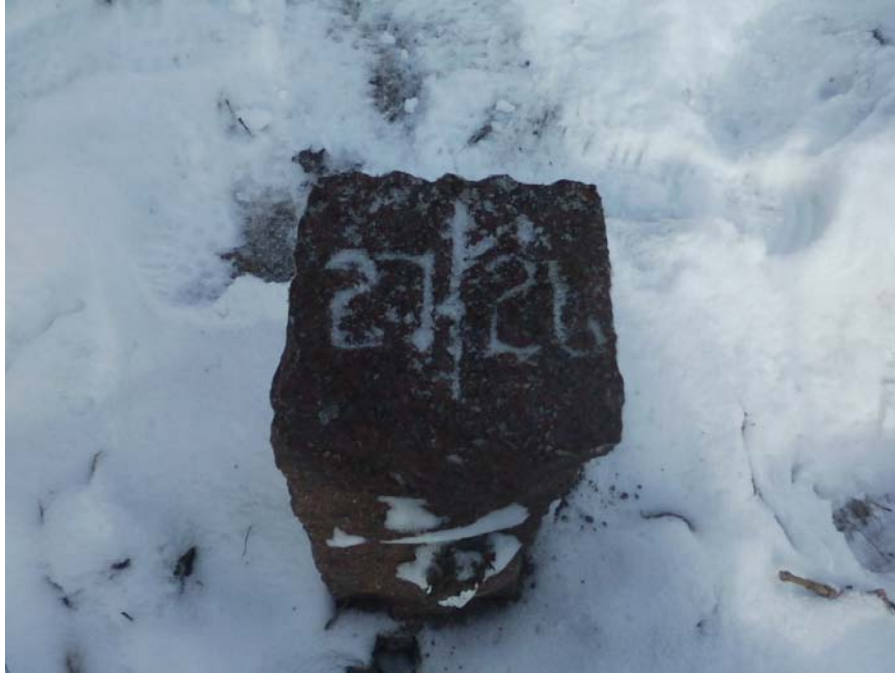
EAST ¼ CORNER, SECTION 27 – 6" SQUARE GRANITE STONE FOUND
