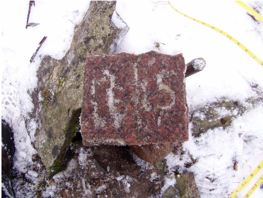
EAST ¼ CORNER, SECTION 16 – 6" SQUARE GRANITE STONE FOUND
