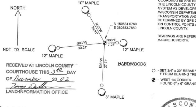
COORDINATES ARE REFERENCED TO THE LINCOLN COUNTY COORDINATE SYSTEM AS DEVELOPED BY THE WISCONSIN DEPARTMENT OF TRANSPORTATION AND WERE DETERMINED BY GPS OBSERVATIONS ON CONTROL POINTS AS SUPPLIED BY LINCOLN COUNTY.
