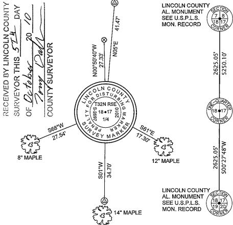
⊗ 1 1/4" DIA. IRON PIPE (STUTH)△ 3/4" DIA. CAPPED REBAR SET
