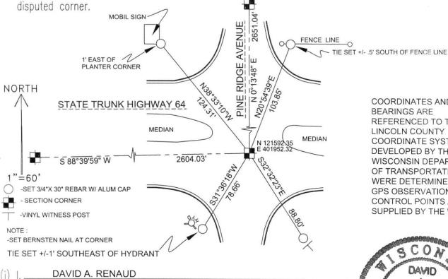
**COORDINATES AND BEARINGS ARE** REFERENCED TO THE LINCOLN COUNTY COORDINATE SYSTEM AS **DEVELOPED BY THE** WISCONSIN DEPARTMENT OF TRANSPORTATION AND WERE DETERMINED BY GPS OBSERVATIONS ON CONTROL POINTS AS SUPPLIED BY THE WDOT.
