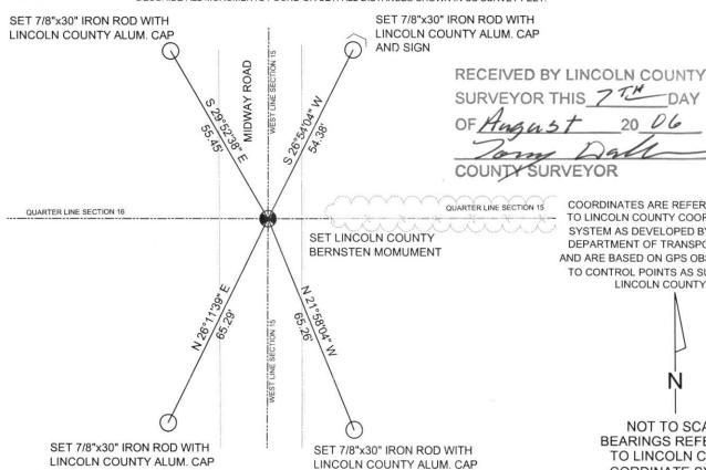
COORDINATES ARE REFERENCED TO LINCOLN COUNTY COORDINATE SYSTEM AS DEVELOPED BY THE WI. DEPARTMENT OF TRANSPORTATION AND ARE BASED ON GPS OBSERVATIONS
