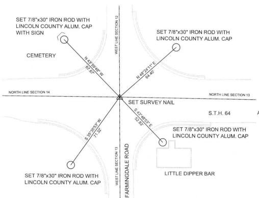
COORDINATES ARE REFERENCED TO LINCOLN COUNTY COORDINATE SYSTEM AS DEVELOPED BY THE WI. DEPARTMENT OF TRANSPORTATION AND ARE BASED ON GPS OBSERVATIONS TO CONTROL POINTS AS SUPPLIED BY LINCOLN COUNTY.
