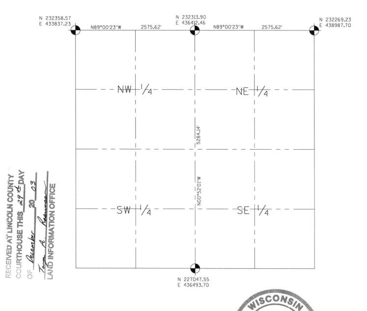
NOTES: COORDINATES AND BEARINGS ARE REFERENCED TO THE LINCOLN COUNTY COORDINATE SYSTEM AS DEVELOPED BY THE WISCONSIN DEPARTMENT OF TRANSPORTATION AND WERE DETERMINED BY GPS OBSERVATIONS ON CONTROL POINTS AS SUPPLIED BY THE DOT.
