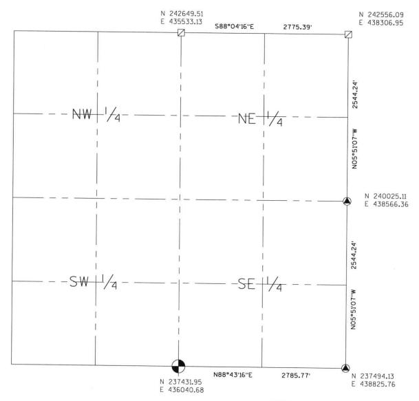
NOTES: COORDINATES AND BEARINGS ARE REFERENCED TO THE LINCOLN COUNTY COORDINATE SYSTEM AS DEVELOPED BY THE WISCONSIN DEPARTMENT OF TRANSPORTATION AND WERE DETERMINED BY GPS OBSERVATIONS ON CONTROL POINTS AS SUPPLIED BY THE DOT.
