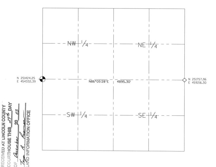
NOTES: COORDINATES AND BEARINGS ARE REFERENCED TO THE LINCOLN COUNTY COORDINATE SYSTEM AS DEVELOPED BY THE WISCONSIN DEPARTMENT OF TRANSPORTATION AND WERE DETERMINED BY GPS OBSERVATIONS ON CONTROL POINTS AS SUPPLIED BY THE DOT.
