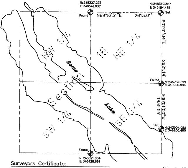
Coordinates and bearings are referenced to the Lincoln County Coordinate System as developed by the Wisconsin Department of Transportation and were RECEIVED BY LINCOLN COUNTY determined by GPS observations on Control Station
