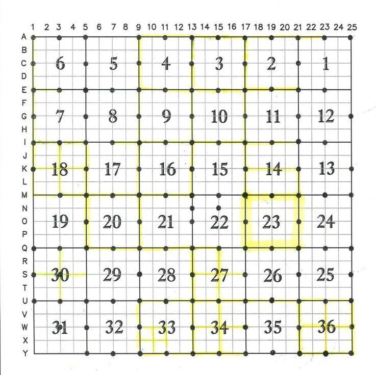
= Corner monumented and record contained herein. Corners such as meander corners which are not located at intersecting lines on the above diagram are identified by reference to adjoining applicable coordinate lines. EX: AB-1, QR-19, S-18,19
