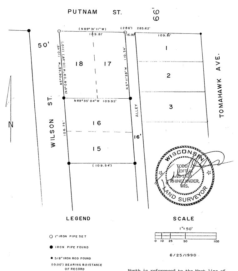
North is referenced to the West line of Block 1 being a recorded bearing of N 5 08 09 W.
