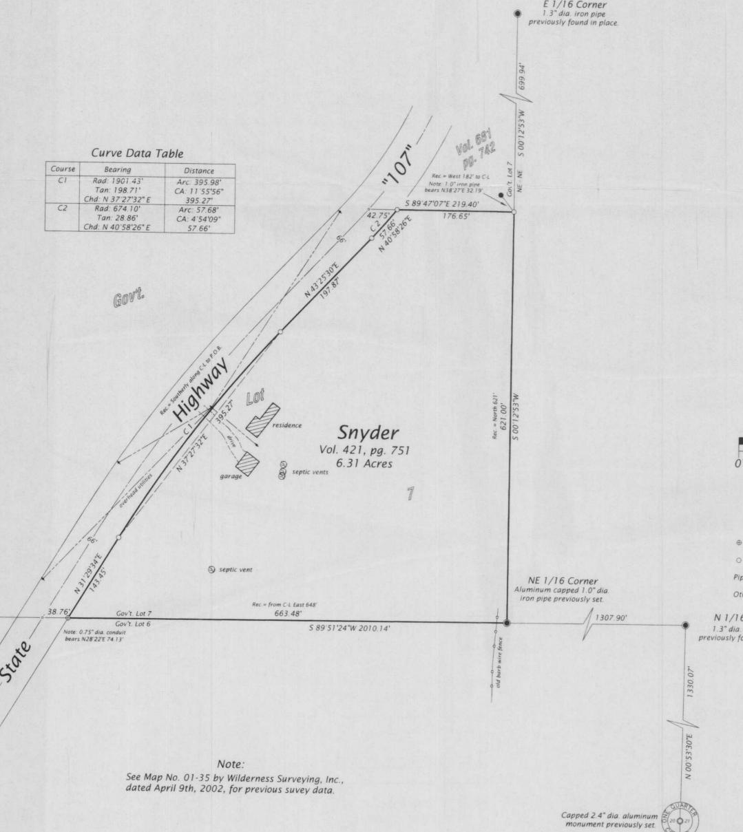
Bearings Lincoln County Grid, based on GPS survey data.
