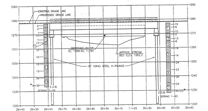
\* THE BLOWS PER FOOT AT THE LOCATIONS INDICATED ARE BASED ON DRIVING A 2" O.D. SPLIT BARREL SAMPLER WITH A 140 LB. HAMMER HAVING A FREE FALL OF 30 INCHES. THE BLOW COUNT IS TAKEN IN UNDISTURBED SOIL BELOW A CASED HOLE ELIMINATING SIDE FRICTION ON THE DRIVE PIPE.
